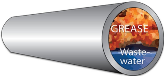
Grease is one of the leading causes of sewer clogs and overflows.
